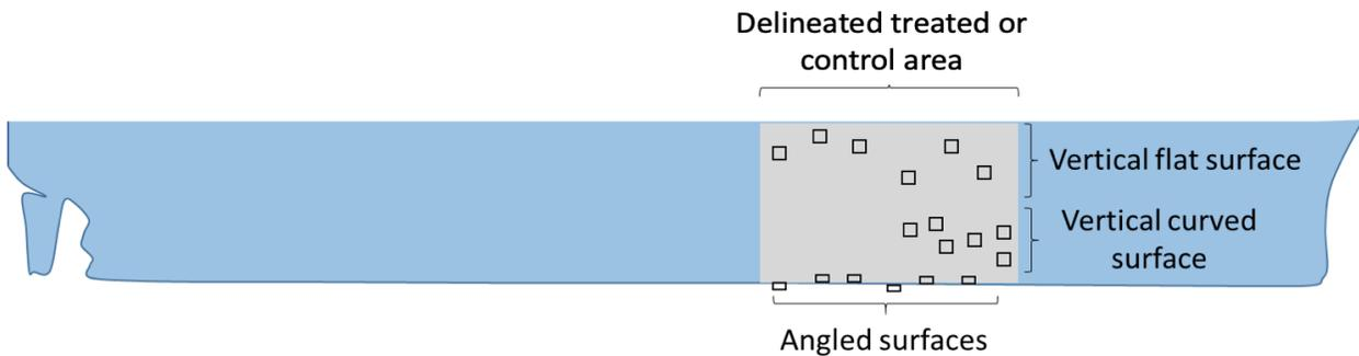
**Figure 3.** Pictorial representation (not to scale) of an example delineating a treated or control area (grey), surface types within the test area, and a stratified, randomized six replicate plots within each surface stratum (black squares). The bottom area, not visible in this figure, should also be sampled using six replicate plots.
