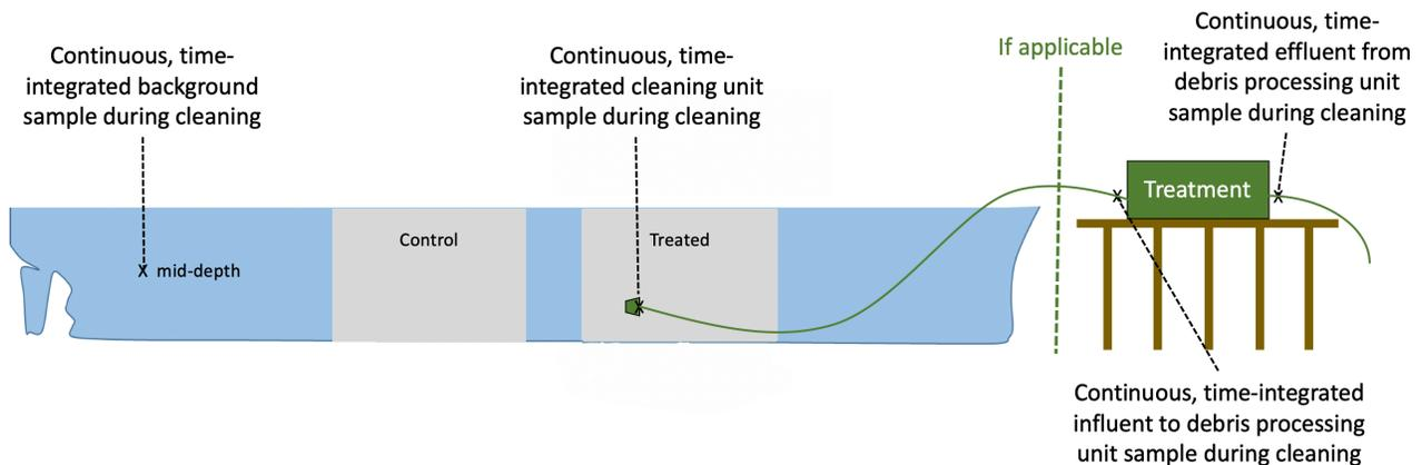
**Figure 6.** Pictorial representation (not to scale) of water quality sampling locations during a test cleaning event. Debris processing and effluent impacts are described in Section 6. Not pictured are the discrete samples of background/ambient conditions taken before and after a test trial at the same location.
