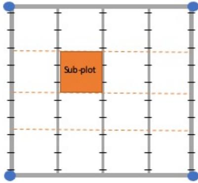
**Figure 2.** Example of a quadrat frame containing four survey bands used to survey each 1 m<sup>2</sup> plot. A total of 16 sub-plots (bounded by the dashed lines between bands) can be imaged and/or 50-point counts defined. Blue circles represent magnets to attach the quadrat for sampling.
