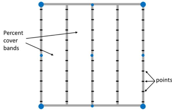
**Figure 6.** Example of a 1 m<sup>2</sup> quadrat that should be used to determine biofouling cover in low visibility conditions.
