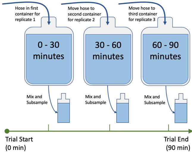
**Figure 7.** Pictorial representation of three-replicate, continuous, sequential, time-integrated water quality sampling, at each sample location, during a test cleaning event.
