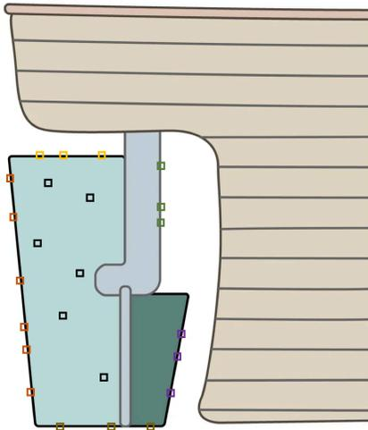
**Figure 4.** Pictorial representation (not to scale) of an example delineating a treated or control niche area, and sub-niche areas. In this example, one side face of the rudder can be treated/cleaned and the other designated as the control. The randomized three to six replicate plots within each sub-niche area of the rudder are designated by different colored squares.
