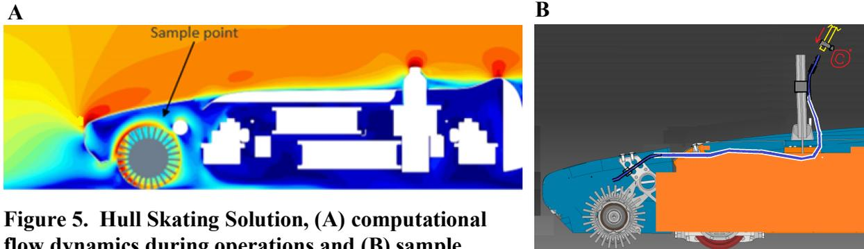
**Figure 5. Hull Skating Solution, (A) computational flow dynamics during operations and (B) sample collection location and design for Station U**
