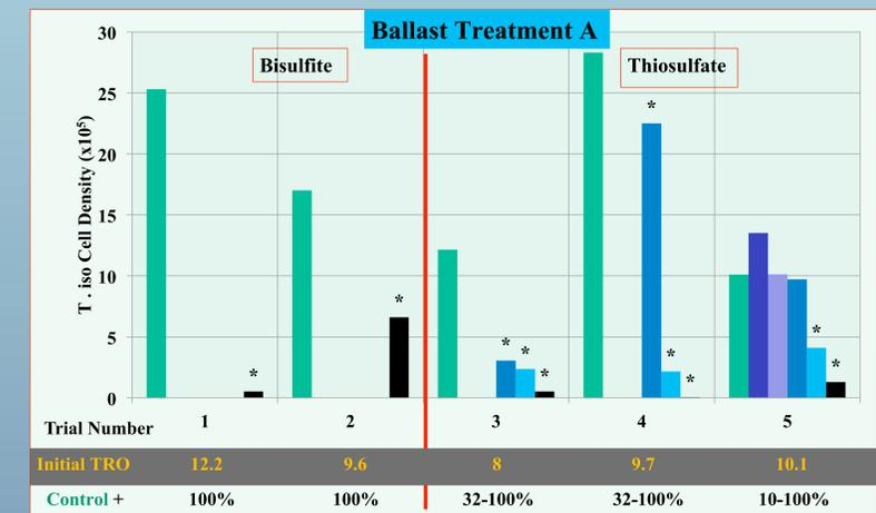
**Figure 4.** Algal toxicity (T. iso) of ballast water (5 trials) that has been chlorinated (electrochlorination), and de-chlorinated (sulfur compounds) after 5 days in ships ballast. Final TRO < 0.02 mg/L. \* Statistically different from control.
