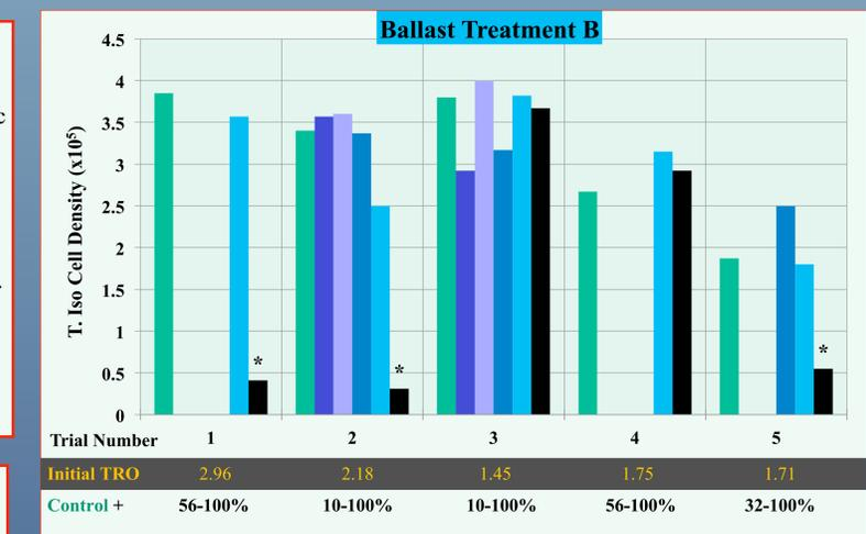
**Figure 5.** Algal toxicity (T. iso) of ballast water (5 trials) that has been chlorinated (electrochlorination) at a low level (1.4-3.0 mg/L) and held for 5 days. Final TRO < 0.02 mg/L. \* Statistically different from control.
