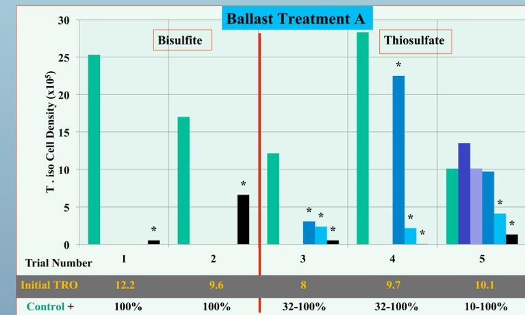
**Figure 4.** Algal toxicity (T. iso) of ballast water (5 trials) that has been chlorinated (electrochlorination), and de-chlorinated (sulfur compounds) after 5 days in ships ballast. Final TRO < 0.02 mg/L. \* Statistically different from control.
