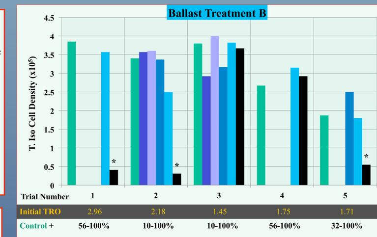
**Figure 5.** Algal toxicity (T. iso) of ballast water (5 trials) that has been chlorinated (electrochlorination) at a low level (1.4-3.0 mg/L) and held for 5 days. Final TRO < 0.02 mg/L. \* Statistically different from control.
