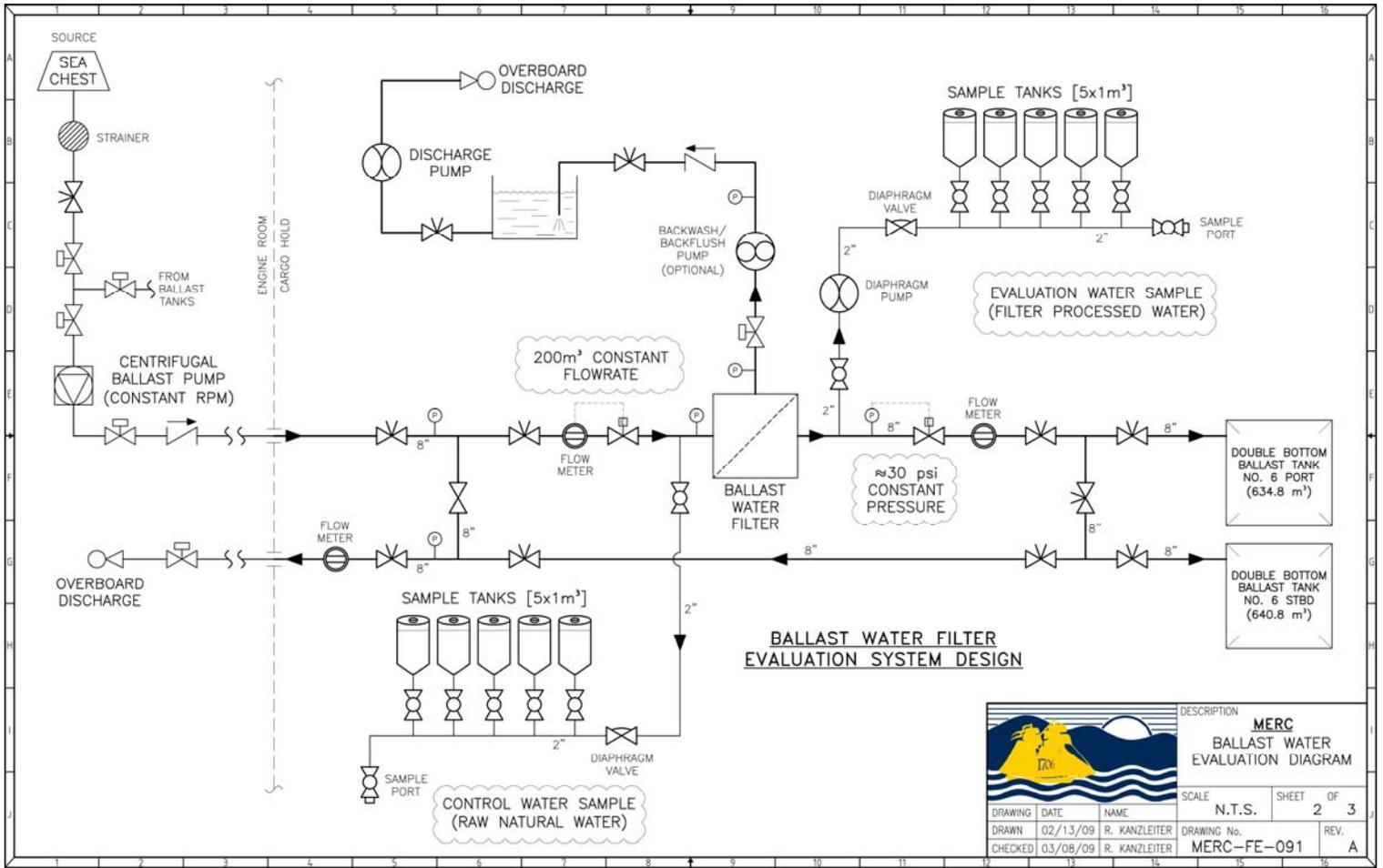
Figure 1. MERC Ballast Water Filter Evaluation System Design
