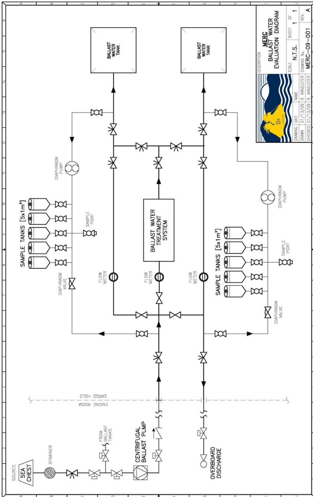
10. MERC Cape Washington ballast water filter system test setup and sampling design.
